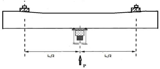
Fig. 4. Schematic set up of negative bending test at center of sleeper
