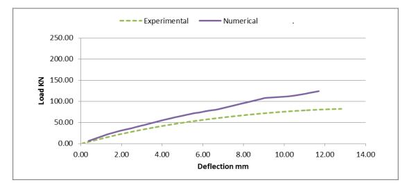
Fig. 19. Load deflection behavior of proposed composite sleeper
