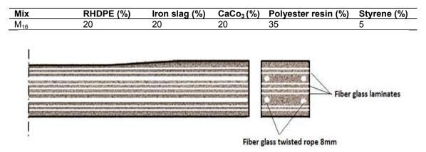
Fig. 2. Reinforcement of full scale proposed composite sleeper
