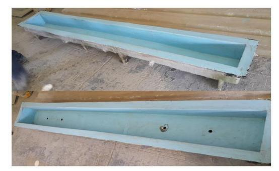
Fig. 1. Mold of proposed composite sleeper
