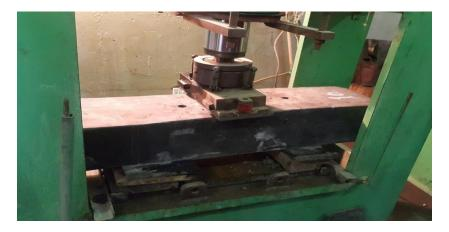
Fig. 7. Actual set up of positive bending test at rail seat position
