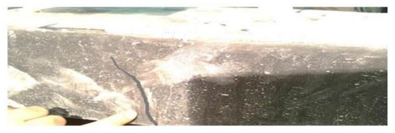
Fig. 10. Failure mode of sleeper S<sub>10</sub> under static load on rail seat section
