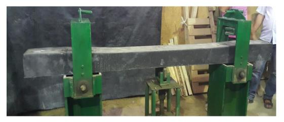
Fig. 5. Actual set up of negative bending test at center of sleeper
