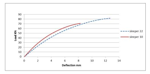
Fig. 8. Load deflection relationship of negative bending test at center of sleeper
