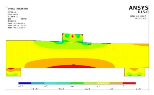
Fig. 13. Composite sleeper stresses at cracking load (N/mm<sup>2</sup>)
