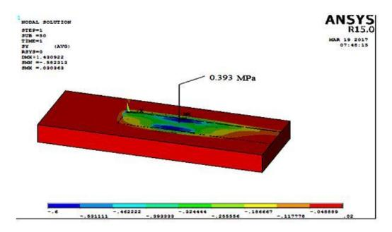
Fig. 22. Composite Sleeper-ballast contact pressure under 43.4 KN rail seat load [12]
