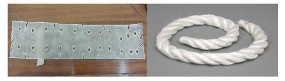
Fig. 3. Used fiber glass laminate and rope in sleeper reinforcement
