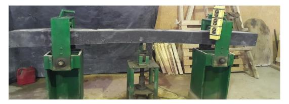
Fig. 9. Sleeper (S<sub>10</sub>) under 72 kN static loading of the sleeper center section
