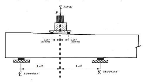
Fig. 6. Schematic set up of positive bending test at rail seat position
