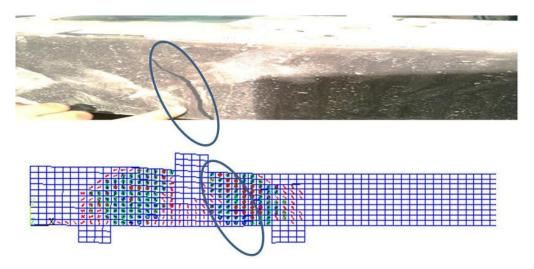
Fig. 15. Cracks expansion at failure
