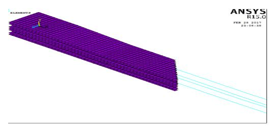
(b) Reinforcing fiber laminates and ropes element; Shell 181 & Link 180
