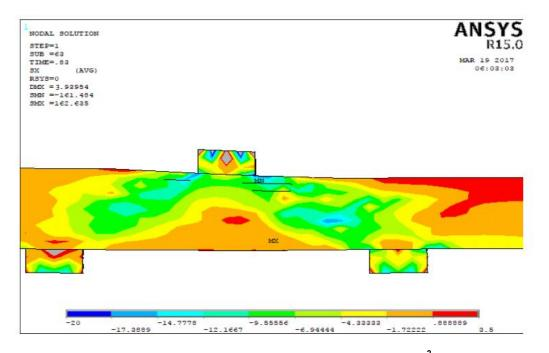
Fig. 14. Composite sleeper stresses at failure (N/mm<sup>2</sup>)
